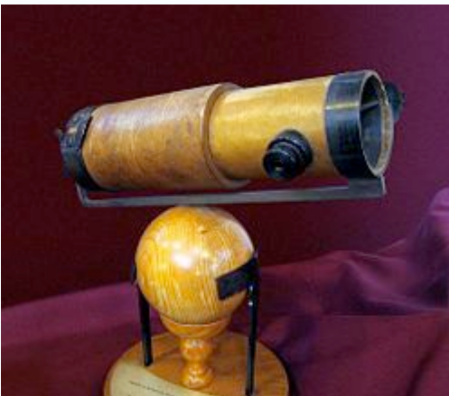
A replica of Newton's 6-inch reflecting telescope of 1672 for the Royal Society.
